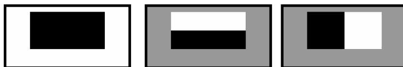
Figure 3.3: The intensity based features used. The absolute intensity difference between the black and the white region is calculated. Left: comparing block to window intensity; right: haar-like edge features
