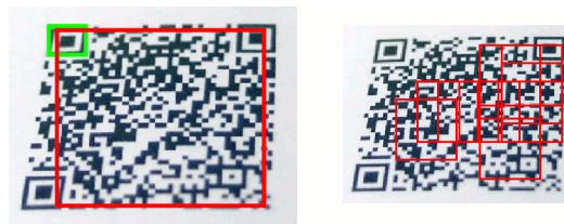
Figure 5.1: QR code labeling (left) and the random square windows used for Adaboost training (right).
