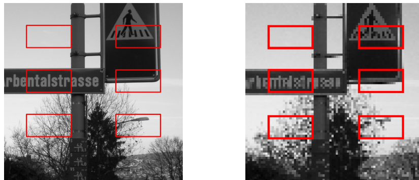
Figure 6.6: The image and feature locations chosen for the scale test. At the smallest resolution, the window has its original size of 20x10 pixels.
