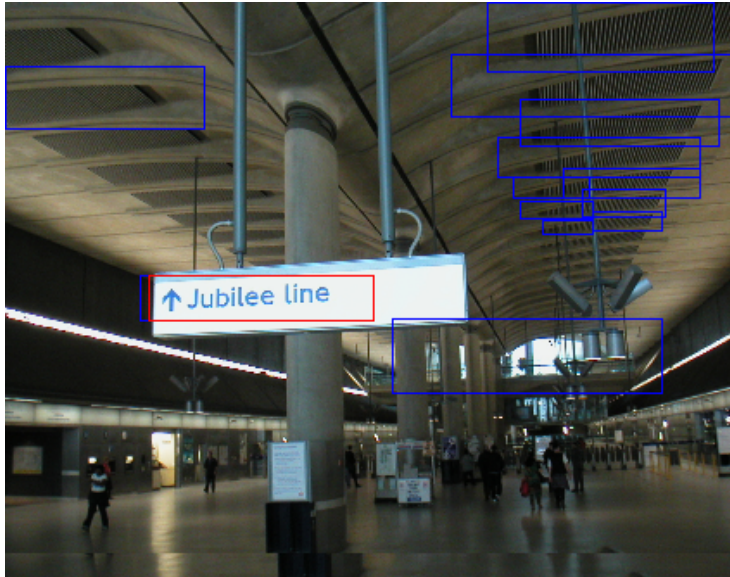
Figure 4.2: Some typical false positives when running at 45e-6 false positives (blue, background). If an image has false positives there are often many of them together, increasing the required OCR processing time a lot. At 5e-6 false positives (red) only the correct text is found.
